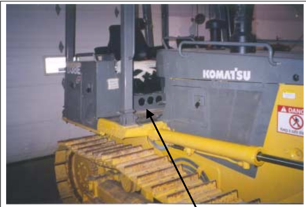
Heater outlets cut in vertical panel of the seat platform
